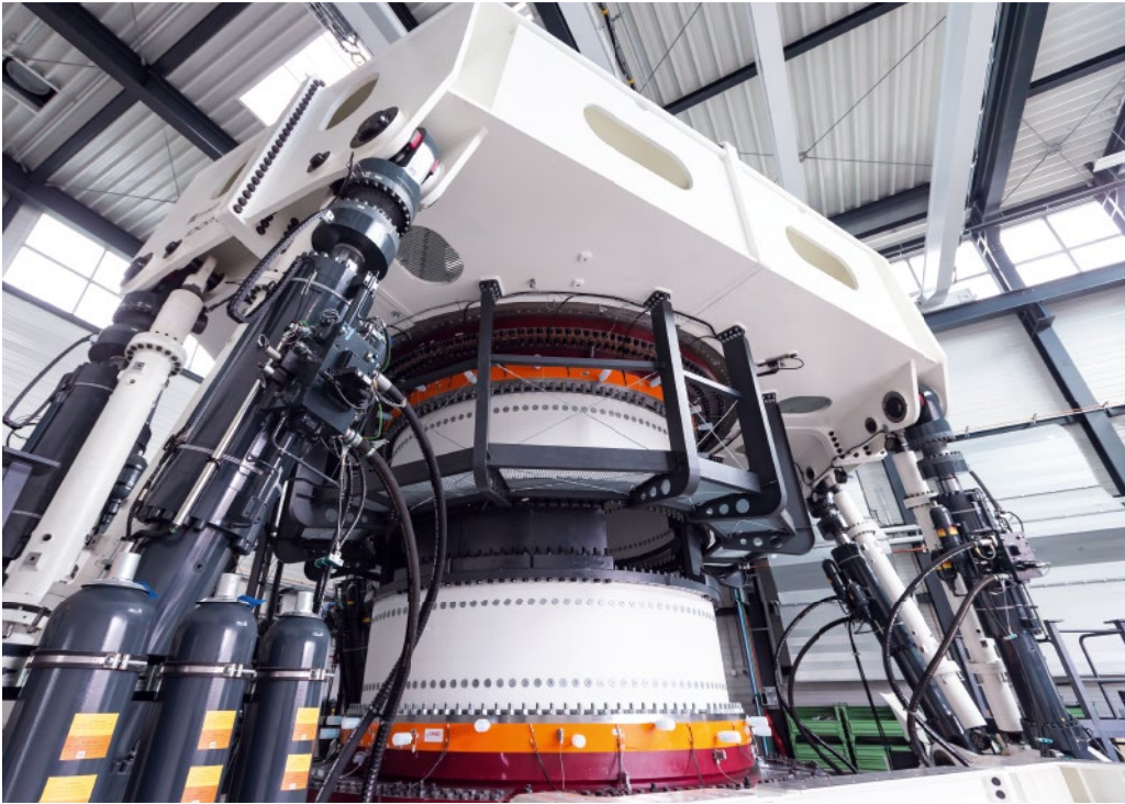
THE HYDRAULIC CYLINDERS IN OUR BLADE BEARING TEST BENCH CAN GENERATE 20 MEGANEWTONS OF FORCE. That is enough to lift three ICE trains at full seating capacity.
